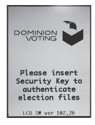
3. Put the iButton (security key) on the Security Keypad.
