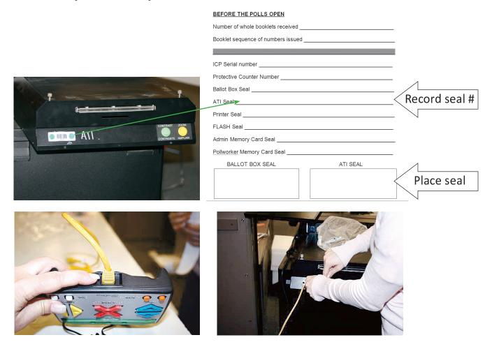
2. Plug headphones into ATI (remote control) under the blue "up and down" arrows.
